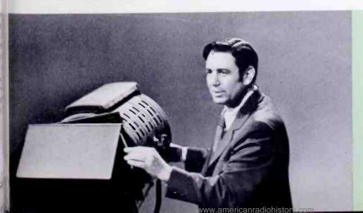
Fig. 3 Barn doors of a spotlight can be used to cut light off at the top, bottom or sides.
