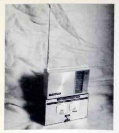
Fig. 1 The simple signal sampler built by the author includes meters for relative signal and modulation readouts.
