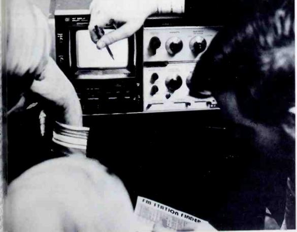
Fig. 2 Author uses local station guide to identify signals on the analyzer.
