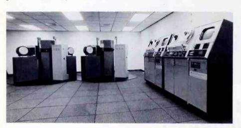
Fig. 2 Film and tape room shown here includes computer flooring and acoustic celling.
