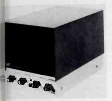
The monitors are available in an tractive single desktop unit or a iple-monitor, 19" rack mount conguration. Entirely manufactured America, the new monitors proide good picture quality and reliaility. A single, plug-in printed ciruit card simplifies maintenance, legulated power supply assures onstant picture size and brightess over a wide range of power ne variation.
